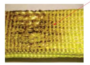
THE DAMAGE: **Knots** compromise the strength of all slings by not allowing all fibers to contribute to the lift as designed. Knots may reduce sling strength by up to 50%.
