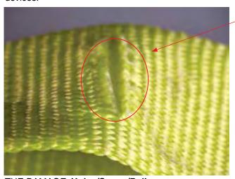
THE DAMAGE: **Holes/Snags/Pulls** WHAT TO LOOK FOR: **Punctures or areas** where fibers stand out from the rest of the sling surface.
